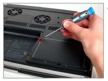
• Remove the 8mm Philips screw located between the hard drive and the WiFi card.
