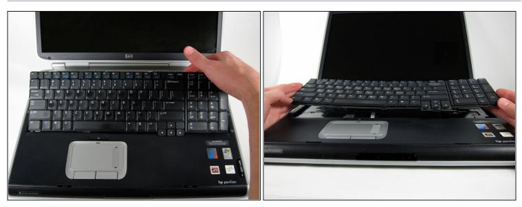
$\triangle$  Lift the keyboard carefully because it is attached to the motherboard by a ribbon cable.
