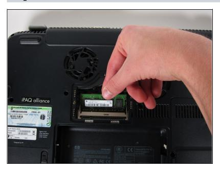
Carefully slide the card out at an upward angle away from the slot.
