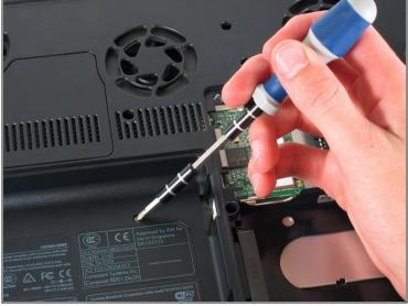
• With the laptop face-down, remove the eleven 8mm Philips screws.
