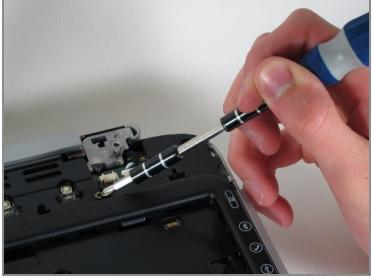
• Unscrew the four 8mm Philips screws from the top cover.
