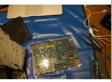
• Gently lift the metal casing from the motherboard. Place it to the side.
