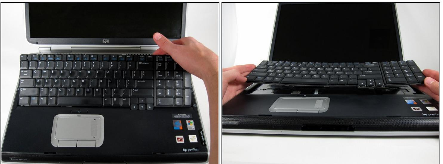
**⚠ Lift the keyboard carefully because it is attached to the motherboard by a ribbon cable.**
