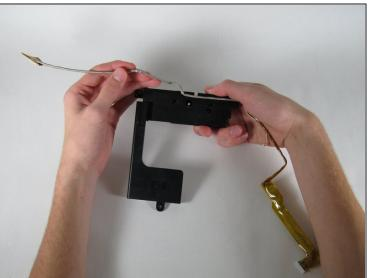
• Lift the speaker unit up, flip it, and remove the USB cable.
