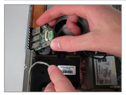
• Pull the module to the right and lift it out to release it.
