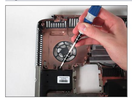
Unscrew the 6mm Philips screw at the back of the left speaker unit.
