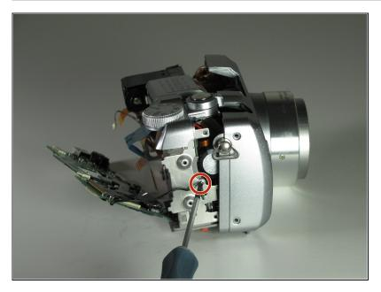
Remove the single 3mm ground screw attached to the right side of the camera body using the Phillips #00 screwdriver.
