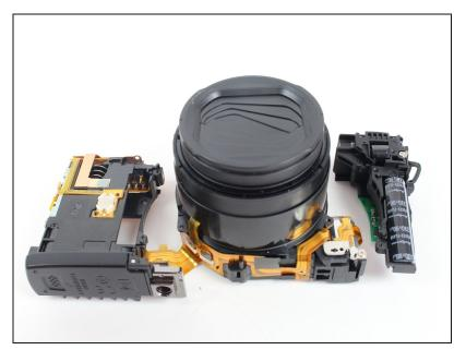
Separate the lens from the other components of the camera.
