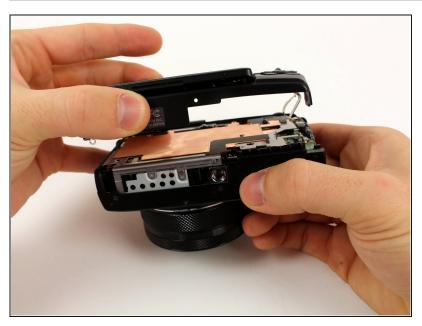
• Carefully lift the back casing away from the camera.
