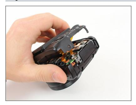
Lift the back casing up far enough to expose the ribbon cables.
