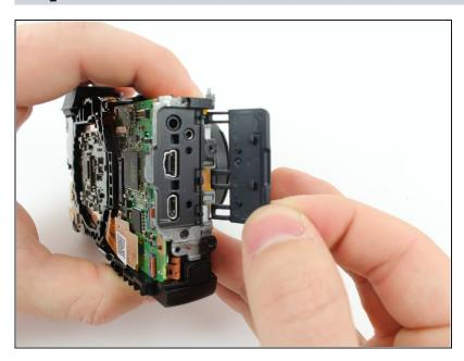
Remove the rubber dust cover from the camera by moving the hooks away from the three prongs holding them in place and then pulling the cover away from the camera.
