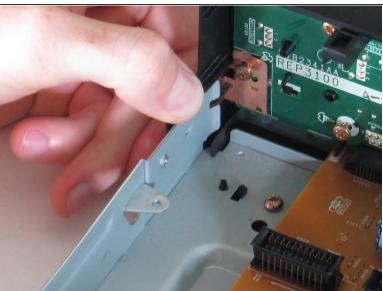
Lift up the five tabs securing the front panel to the chassis. There are three on the bottom, and two
