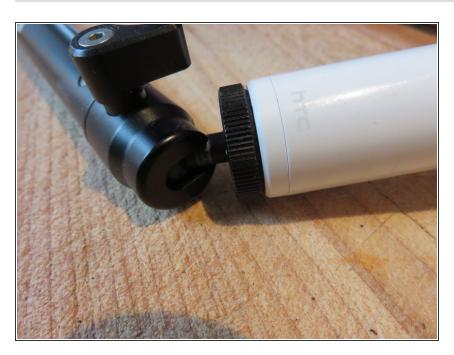
Put a standard camera connection onto the bottom of the camera, so you have something to pull on.
