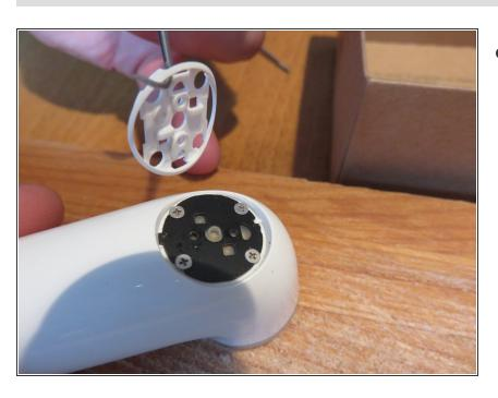
Release 2 black screws to release the button retainer.
