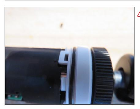
You can see the cap is well locked in place on the main assembly, and worse, as I discovered after breaking it.
