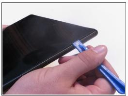
Avoid prying near bottom right hand side due to LCD Connector
