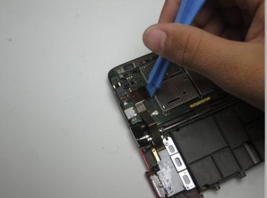
Disconnect the wire with the plastic opening tool.
