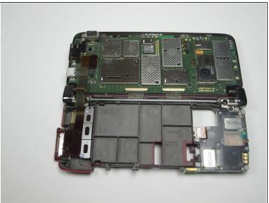
With the screws removed, the sensor board should be free to flip up.
