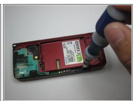
Unscrew the indicated screws using the T5 screwdriver.
