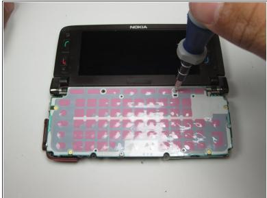
With the T5 Screwdriver, remove the marked screws.
