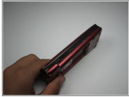
• Using a plastic opening tool, separate the back cover from the phone.
