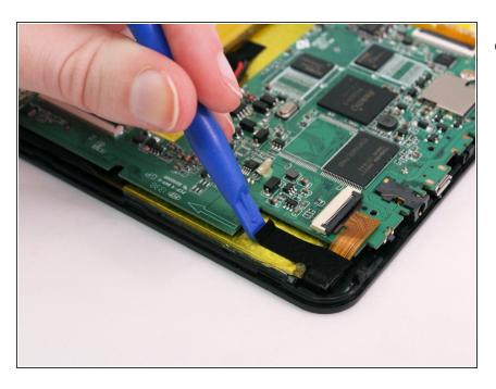
Remove the black tape holding down the ribbon cable.
