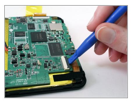
With a spudger, flip up the ZIF connector that connects the camera's ribbon cable to the motherboard. This will release the ribbon cable.
