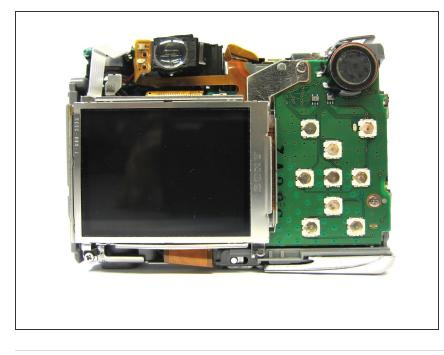
Once the ribbon connecting the back cover is removed, the back of the camera body should look like this.
