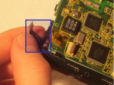
Behind the motherboard remove the brown plastic clamp and remove the front screen cover.
