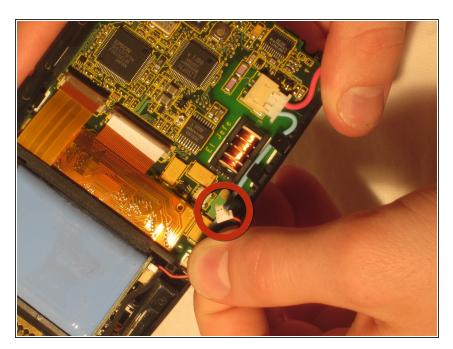
Unhook battery cable from the motherboard and remove the battery.
