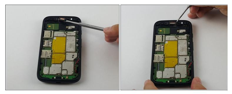
• Using the metal spudger tool, very carefully remove the speaker by first gently prying up on the right side and then the bottom.
