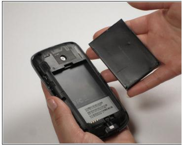
Insert your finger or a pry tool into the slot above the battery. Remove it and set aside.
