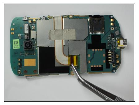
Place the motherboard down on top of the LCD. Using tweezers, remove the yellow piece of tape covering the end of the flat ribbon cable.
