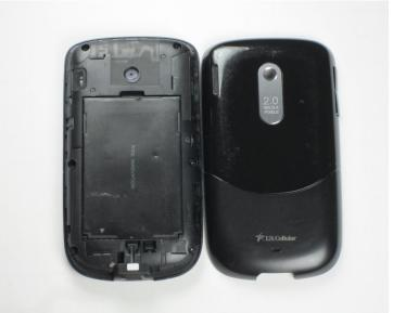
• Using both thumbs, push the back side of the phone's exterior up and remove the front face of the phone.
