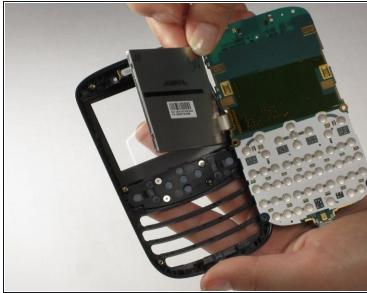
• Using a spudger, remove the display screen from its cell within the front case. Insert the spudger next to the LCD on the opposite side of where the motherboard is attached.
