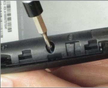
• To remove the case, use a small, pentagonal screwdriver to unscrew the 6 screws that can be found around the edges.
