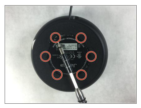
Remove the six 20 mm T6 screws from the bottom of the device.
