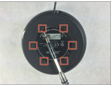
Using a metal spudger, peel back the foam pad on the bottom of the device to reveal six screws.
