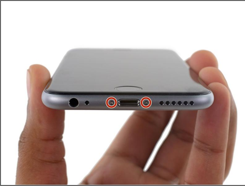
**⚠** Before disassembling your iPhone, discharge the battery below 25%. A charged lithium-ion battery can catch fire and/or explode if accidentally punctured.
