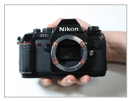
Use a 00 Phillips head screwdriver to remove the four screws from the lens mount.
