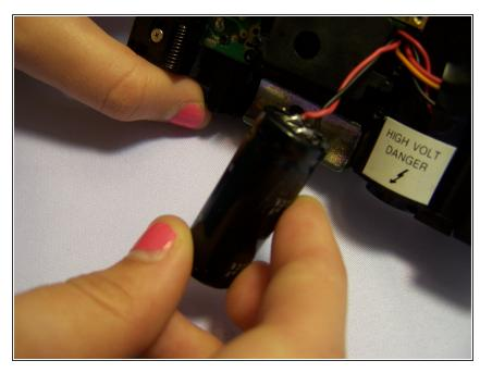
i The capacitor is located at the bottom center of the camera.
