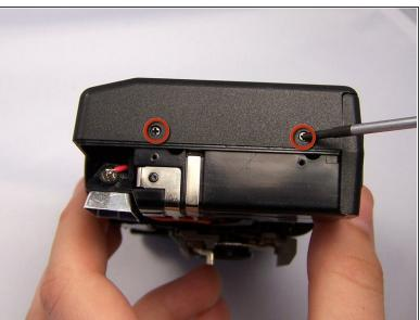
Remove the two 6.2mm Phillips screws on both sides of camera's back cover.
