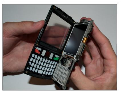
Remove the front faceplate by lifting it off of the phone chassis.
