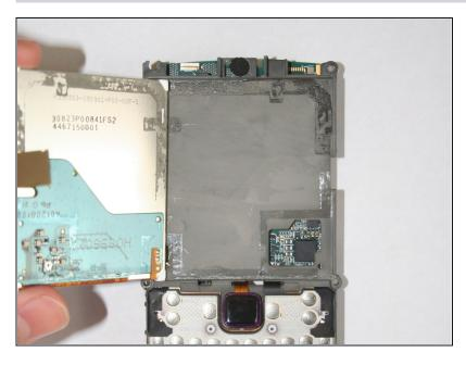
• Lift the LCD display out from phone chassis.
