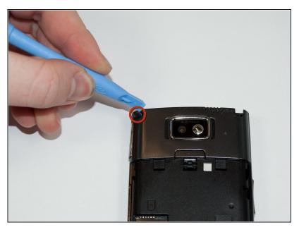
Remove the rubber screw cover in the top left corner by prying upwards with an opening tool.
