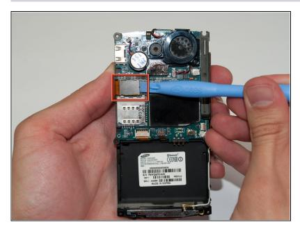
• Using the opening tool, unlatch the LCD ribbon cable.
