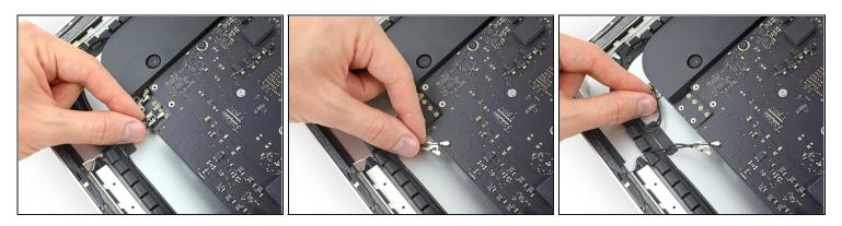
• Gently push the antenna cables aside to clear access to the AirPort/Bluetooth card.
