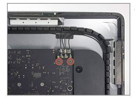
Remove the two 3.3 mm T5 Torx screws securing the AirPort/Bluetooth card to the logic board.
