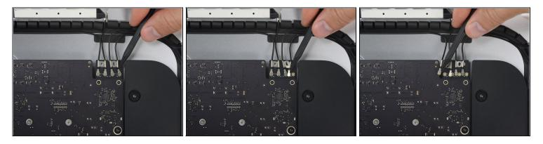
• Use a spudger to disconnect all four antenna connectors by prying them up from their sockets on the AirPort/Bluetooth Card
