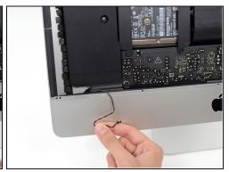
• Gently de-route the power button cable from its groove in the left speaker.
