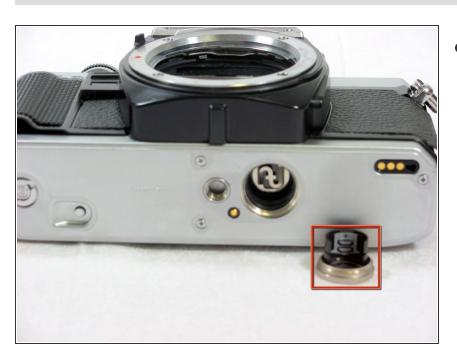
Remove the batteries, making sure to note their proper alignment. To reassemble your device, follow these instructions in reverse order.
