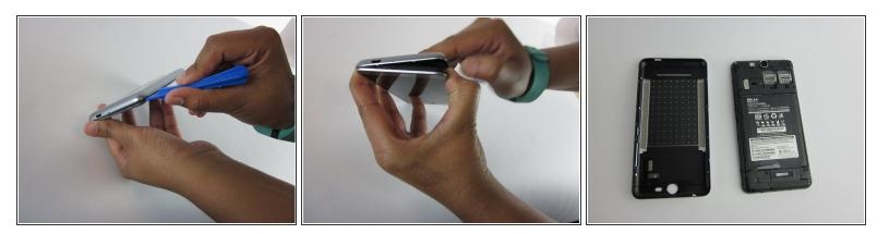
• Pry open and remove back cover with plastic spudger.
