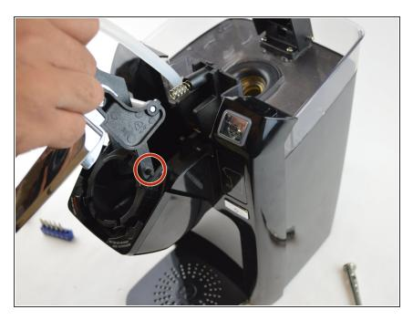
To pull this part off, pull inwards with the these tabs located on both sides of the handle assembly.
