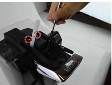
Next, after the removal of the hose on the top by simply pulling it off, remove the following four Phillips #1 screws.
