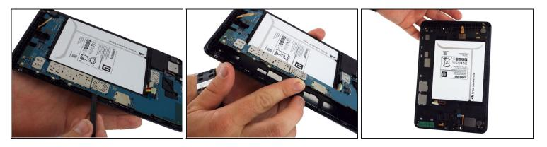
• Using the flat end of a spudger, carefully wedge the motherboard from the case.
