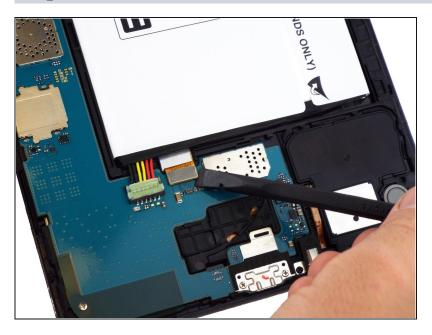
• Use the spudger to disconnect the LCD panel's flexible cable connector.
