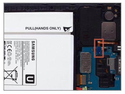
• Use the spudger to disconnect the 3.5mm headset jack's flexible cable connector.
