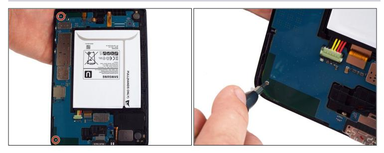
• Use the PH0 screwdriver bit to remove the two 3 mm screws on the left side of the motherboard.
