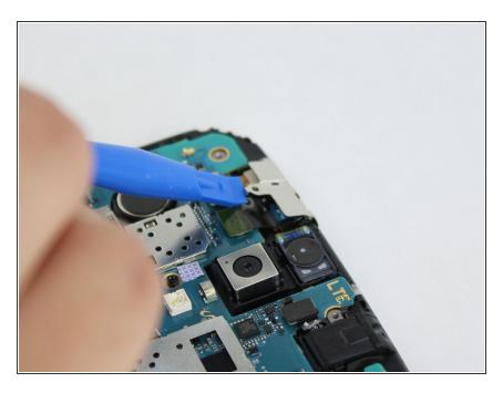
Remove the metal cover with the plastic opening tool.
