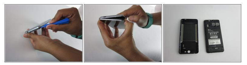
• Remove the back case using plastic opening tool.
