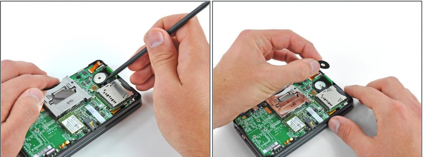
ⓘ To decrease the chance of losing it during repairs, you may want to remove the two thin pads underneath the Circle Pad joystick.
