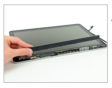
Remove the clutch cover from the display.
