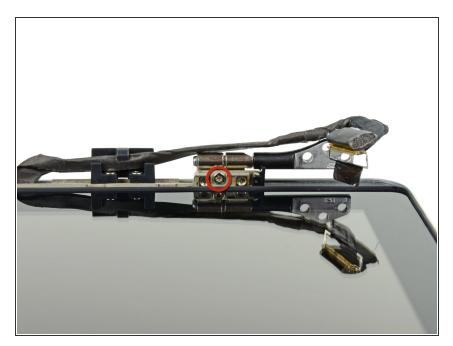
Remove the single 5.2 mm T6 Torx screw securing the left clutch hinge nearest the display glass.
