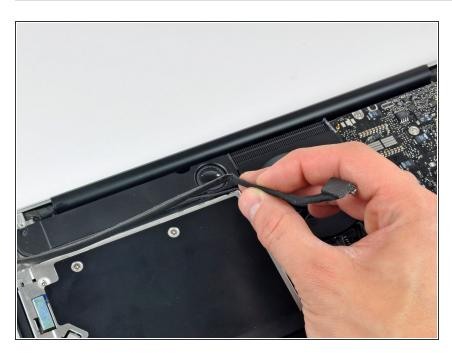
De-route the camera data cable from the channel in the optical drive.
