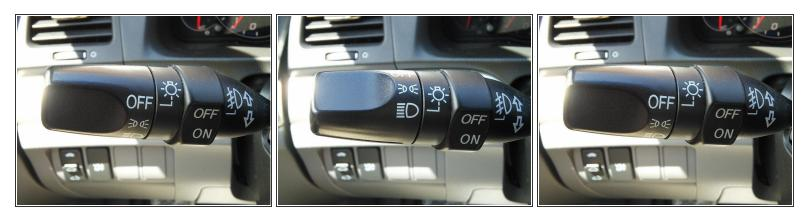
• Within five seconds, and still holding in the **Sel/Reset** button, turn the headlights OFF, then ON, then OFF again.
