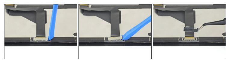
• Use an opening tool to pry up one end of the EMI shield covering the second display cable.
