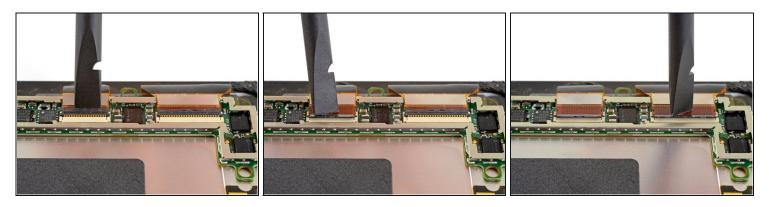
• Use a spudger to flip up the small locking flaps on the display cable ZIF connectors.
