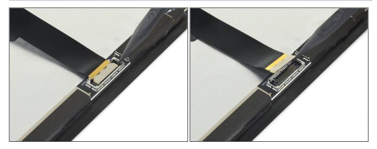
• Use the tip of a spudger to pry the digitizer connector straight up and out of its socket on the screen.
