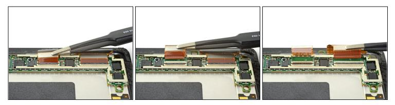
• Use tweezers to slide the display cables straight out of their sockets on the display board.
