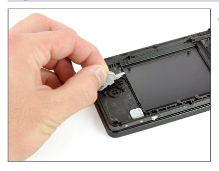
• Peel the grey silicone cover off the back of the ABXY buttons.
