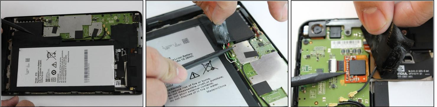
**⚠** Be careful when removing the two pieces of tape because there are wires underneath the tape. Lifting too hard may accidentally rip out the wires.
