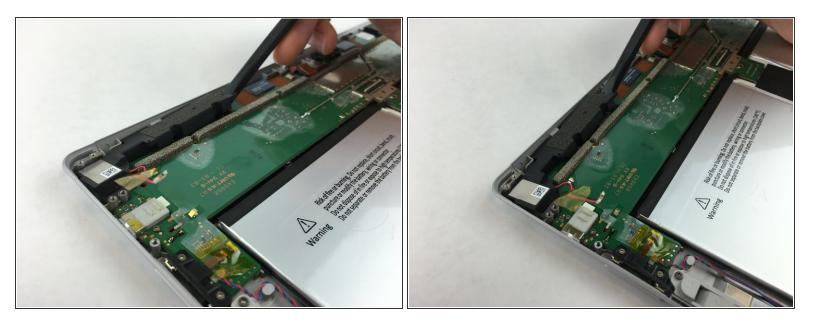
Lifting from the inmost end of the speaker, use a spudger to carefully pry the speaker from the motherboard.
