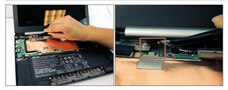
Disconnect the black and white cables located near the screen hinge.
