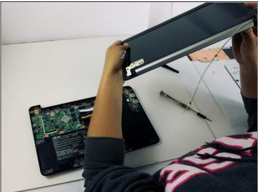
• Carefully pop the LCD screen assembly out of the laptop case.
