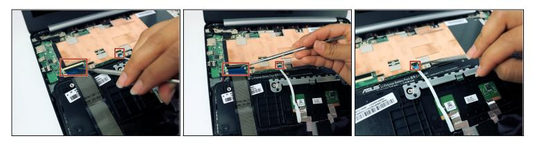
Use the metal spudger to gently pry up the small tabs that are clamping down on the keyboard cables.
