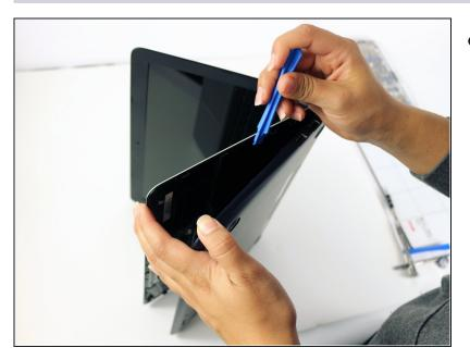
Turn the laptop on its side. Use a small, blue opening tool to pry the keyboard cover and laptop apart. Begin from the top right, next to the power button, and slowly work your way around to the opposite side until the keyboard cover is detached.
