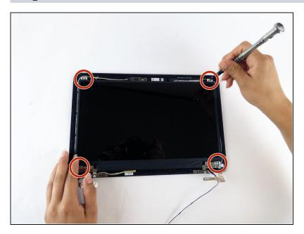
Remove the 4, 3mm silver corner screws holding in the LCD.
