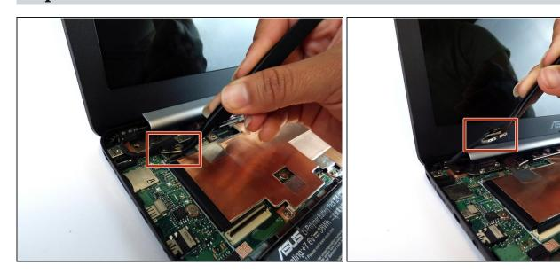
• Locate the LCD cable and its connector which is located in the upper left hand corner of the computer. Carefully flip up the tiny tab and safely remove the cable using precision tweezers.
