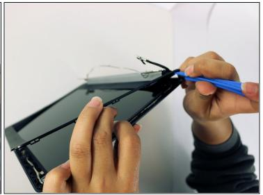
• Use a blue plastic spudger to snap the LCD cover off, working the spudger around the perimeter and completely remove the cover.
