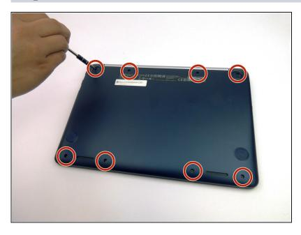
Use the J0 screwdriver to remove the eight 5mm black screws on the bottom of the laptop, which includes the two that were hidden under the rear rubber feet.
