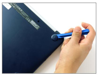
Remove the two rear rubber feet by using one of the small, blue plastic spudgers.
