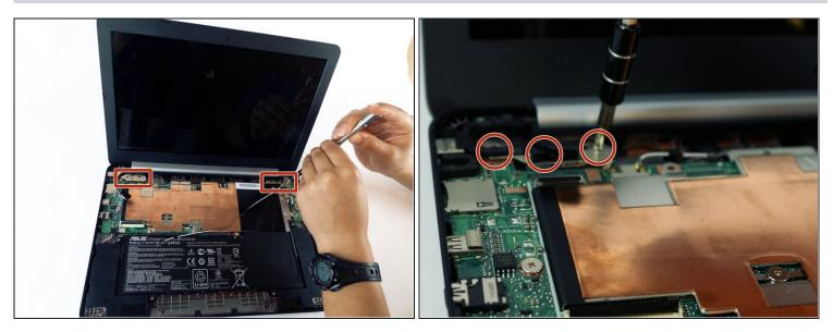
• Remove the 6, 4mm silver screws from the hinges attaching the LCD to the laptop using the J0 Phillips screwdriver.
