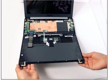
Gently flip the keyboard cover away from the laptop. Rest it safely upside down so the cables are not strained and are easily accessible.
