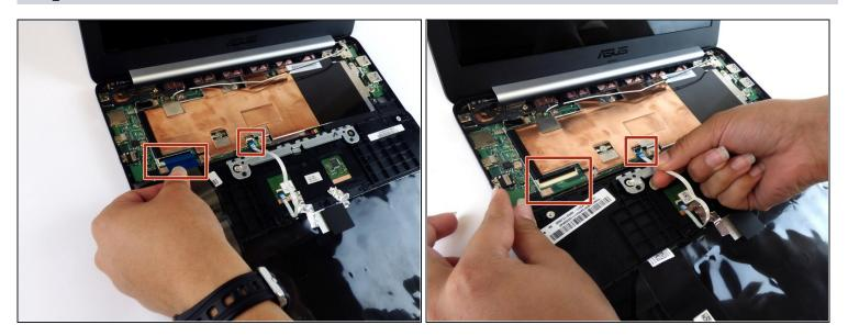
• Carefully pull the keyboard cables out of the connecting ports that are attached to the motherboard.
