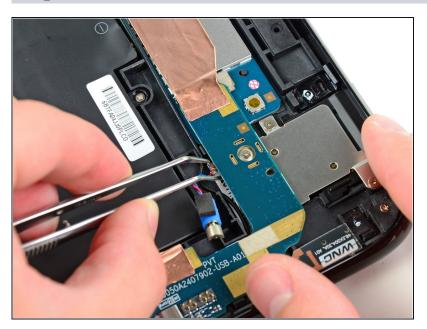
Pull the vibrator motor connector straight away from its socket on the USB connector board.
