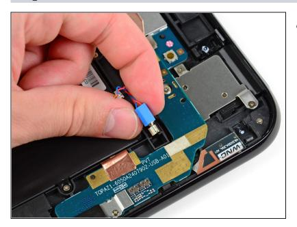
• Remove the vibrator motor from the rear case.
