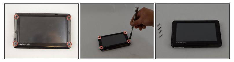
• Remove the four 11.0 mm screws using the Torx T5 screwdriver.
