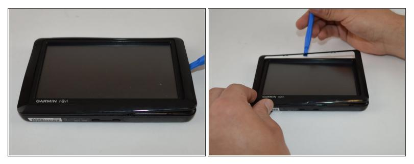
• Slide the plastic prying tool around the perimeter to completely remove the frame.
