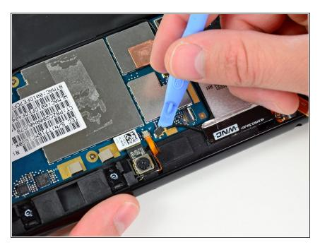
Use a plastic opening tool to pry the upper antenna connector up from its socket on the motherboard.
