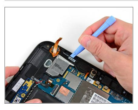
Use a plastic opening tool to peel the upper antenna off the adhesive securing it to the top speaker.
