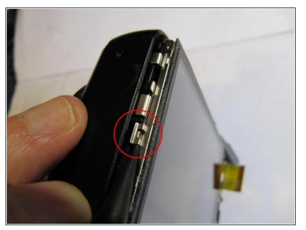
Release a clip on the left hand side of the LCD and hence lift the LCD out.
