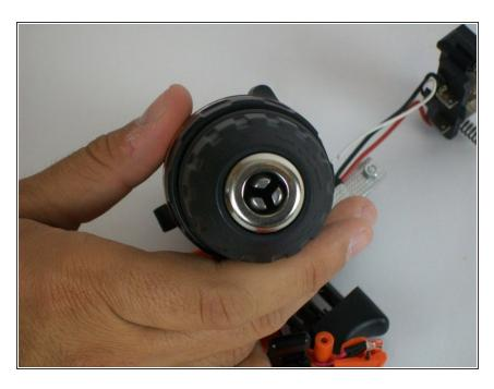
The three metal tips in the front are the ones that are controlled by the chuck to hold and release the screw.
