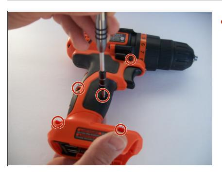
Remove the five screws on the front side of the drill.
