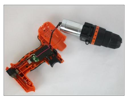
While separating the top from the rest, do this carefully without over stretching the wires so that no connection is damaged.
