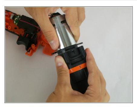
To remove the motor simply twist as illustrated in the picture.
