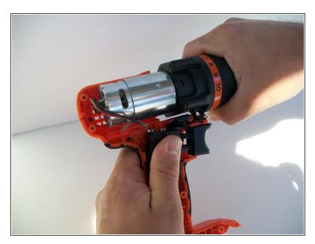
Separate the top part(the chuck and motor) from the rest of the drill.
