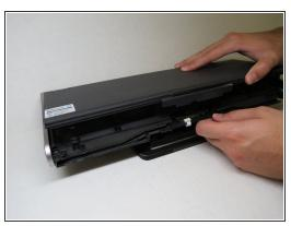
With the front of the speaker facing you, run the plastic opening tool along the bottom of the speaker. Then push the face of the speaker at both ends before lifting it off.
