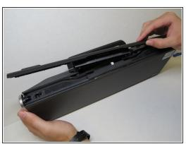
Use the plastic opening tool to run along the outside edges of the speaker. Pry along the seams until you can remove the side panel of the speaker, exposing the battery.
