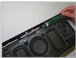
Lift off the casing on the left, right, and top of the speaker.
