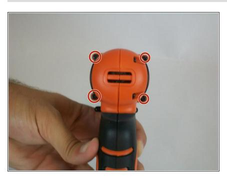
Remove the four screws on the back top side of the drill.
