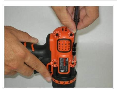
Remove the four screws that connect the chuck to the drill.
