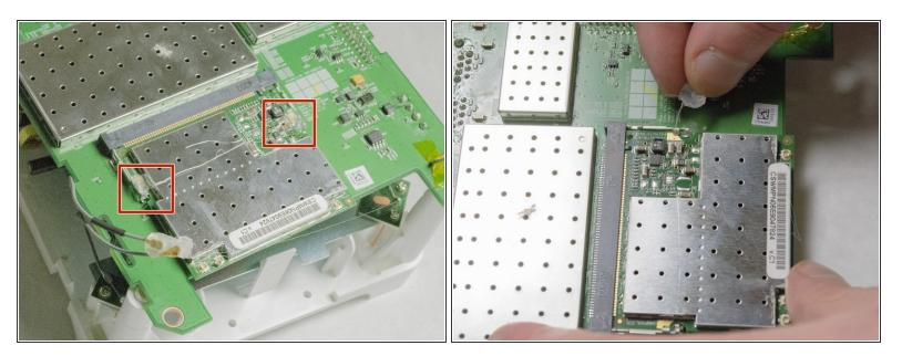
• Remove the two pieces of glue holding the WIFI card in place.
