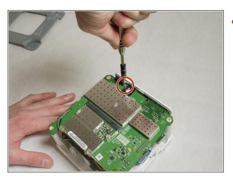
Remove the 7mm length Phillips screw holding the board in place.
