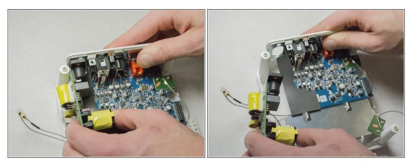
• Pull the power supply out of the back of the device.
