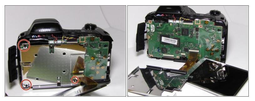
In order to get to the motherboard to disconnect the old LCD screen, you need to remove three 5 mm Phillips #000 screws that connect the bracket piece to the motherboard.
