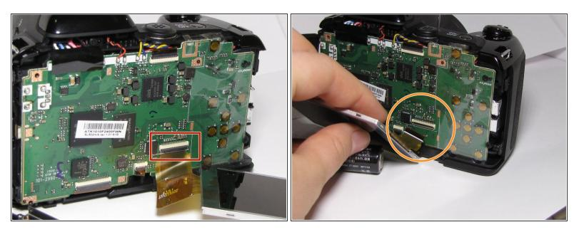
To remove the old LCD screen from the motherboard, there is an off-white ribbon on the motherboard that, the thin black ZIF (Zero Insertion Force) connector that needs to be lifted up so that the circuit piece connected to the LCD screen can be pulled out.
