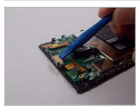
Remove USB port cover using the plastic opening tool, or your hand. It can be removed easily.
