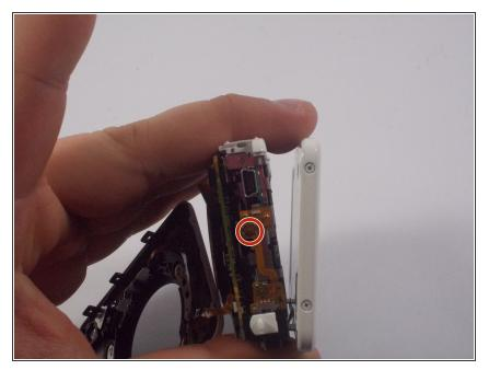
• Flip over and remove 1 screw from side with playback/phone options .
