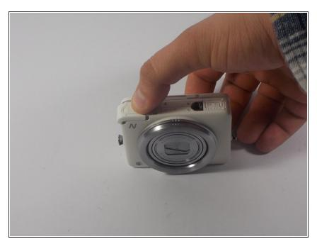
• Place finger on the textured portion of battery housing cover and slide cover in the direction indicated.
