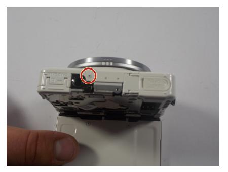
• Remove one screw from the bottom of the camera.
