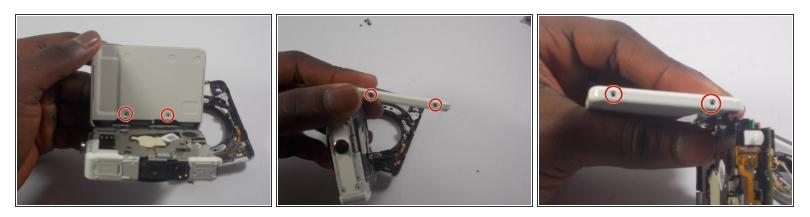
• Unscrew 2 screws from top, bottom, and both sides of screen.
