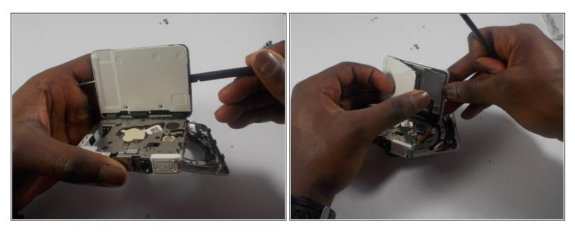
• Remove white metal plate behind screen (tip: try not to bend).
