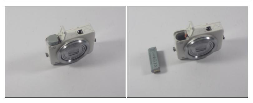
• Remove battery from battery slot with fingers.
