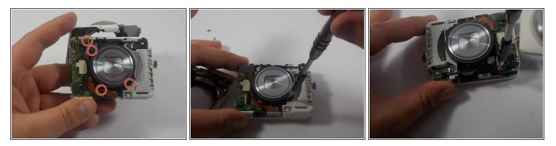
• With the camera lens facing you, remove 4 screws around the lens.
