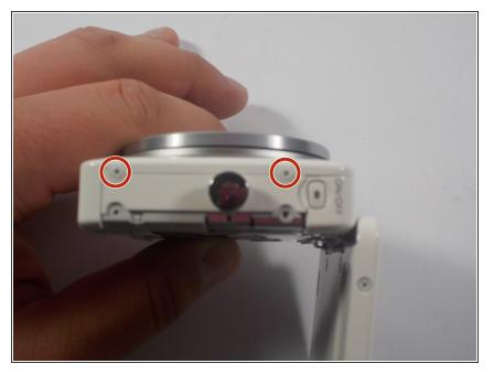
• Locate 2 screws on "on/off" side of the camera and unscrew them.
