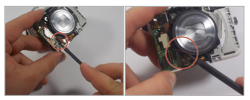
• Using plastic spudger, push tab to release the ribbon cable.
