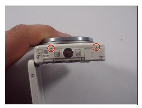
• Locate 2 screws on the other side of the camera and remove them.
