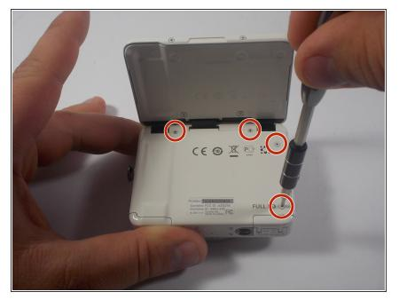
Using a PH000 size screwdriver, unscrew four screws beneath screen.
