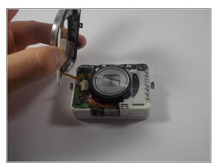
Remove front plate from motherboard so that one ribbon cable is exposed.
