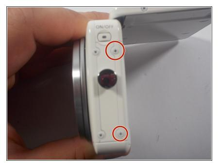
Remove 2 screws from the side of the camera with the on and off buttons.
