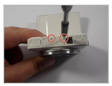
• Remove 2 screws on the bottom of the camera.
