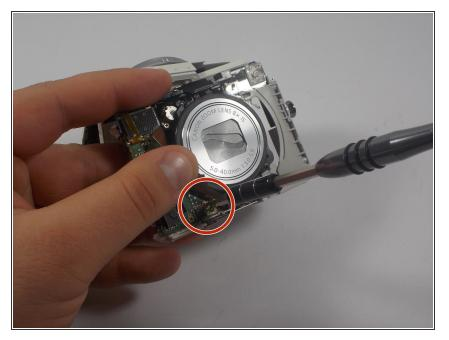
• Locate screw under released ribbon cable and remove it.
