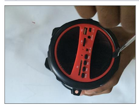
• Use a metal spudger to remove the mesh speaker covers (the side with the buttons) by wedging the narrow end into the center of the outer edge of the mesh, touching the red plate.
