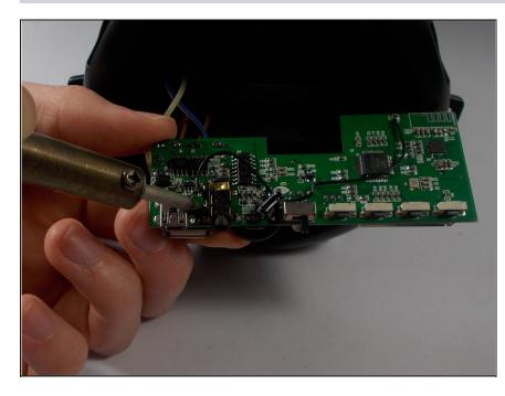
• To remove the port, heat up 5 different solder points using a soldering iron.
