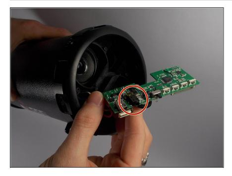
• Locate the auxiliary port which is on the left side above the USB drive and to the right of the charging port (auxiliary port has a circular front).
