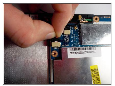
Disconnect the power component from the motherboard by pulling it out horizontally. Do not pull up on the cord only pull out
