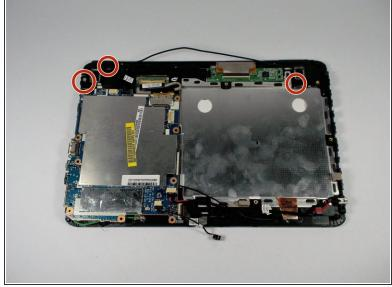
After removing the battery use a Phillips head #00 screwdriver to remove the 3.0 mm screws holding the dual speakers in place.
