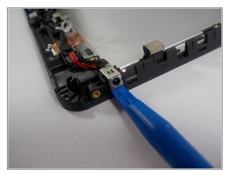
Using the plastic opening tool gently lift up the charging component out of its slot in the case.
