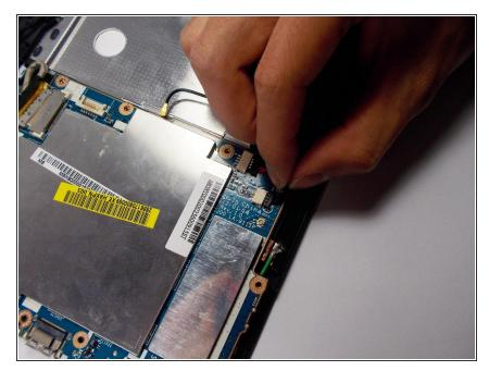
Once the microphone has been lifted away from the case, disconnect the microphone cable from the motherboard by pulling the cable out horizontally. Do not lift up to remove.
