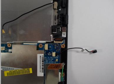
Lift up on the microphone cable to lift the microphone component away from the case.
