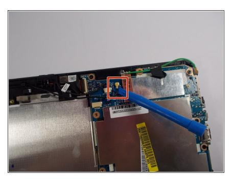
Using the plastic opening tool unplug the black cable by placing the tool under where the cable meets the plug and lift up.
