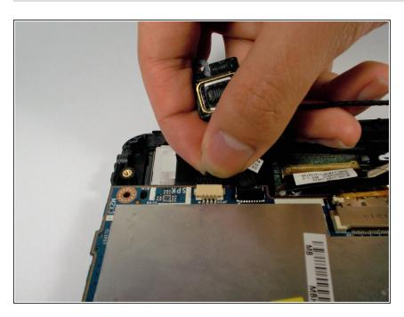
Once you have removed the speakers from the case, disconnect the speakers from the motherboard by pulling the cable out horizontally. Do not pull up on the cable.
