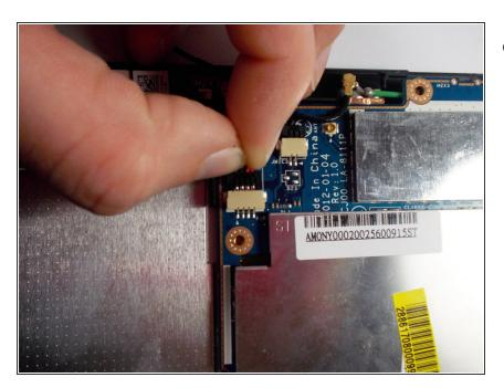
Disconnect the power component from the motherboard by pulling it out horizontally. Do not pull up on the cord only pull out
